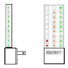
Powerkuff® Grid Monitor showing 28,900 watts in use, Each Column red 10 Kw, amber 1Kw, and green 100 watt
